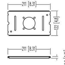
**FLANK CAP WITH 60 MM (2.36") DIAMETER OPENING (OPTIONAL)**
